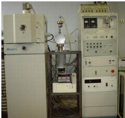
*High-frequency magnetron sputtering facility*
