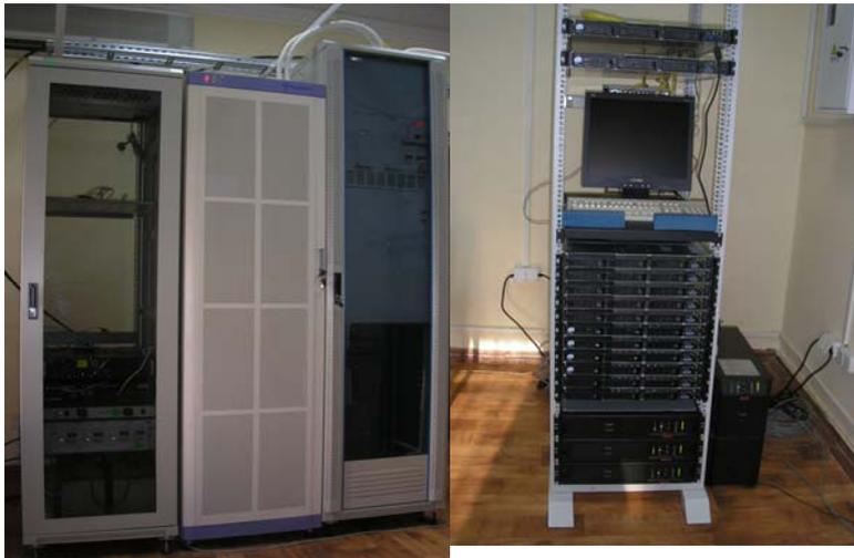
The IAP Cluster is a beowulf cluster comprising 11 computational and one master node. There are 88 processor cores, wide variety of software and compilers that support MPI and OpenMP standards available for users. For cluster load control a queuing system Torque is used.
