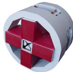
*A new type of active ion-optical element, an integrated doublet or quadrupole lenses*
