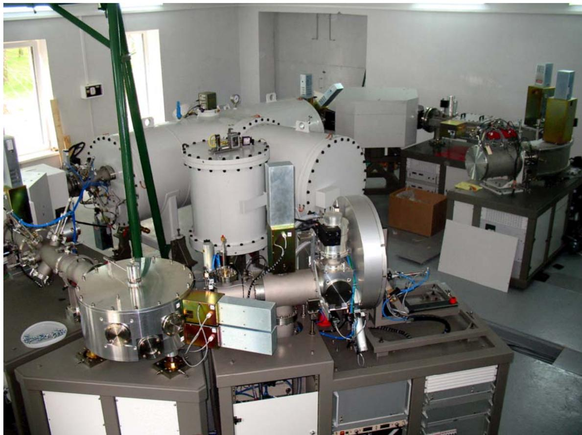
AMS facility (model 4110Bo-AMS) is a 1 MV Tandetron, multi-element machine designed to be able to detect not only low-mass isotopes such as  $^{10}\text{Be}$ ,  $^{14}\text{C}$  and  $^{26}\text{Al}$ , but also heavy elements such as  $^{129}\text{I}$ . This type spectrometer was used to analyze the Shroud of Turin.
