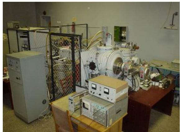
*High-intensity ion source testing equipment*
