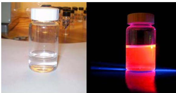
Colloidal solutions of \text{GdVO}_4:\text{Eu}^{3+} nanocrystals (left ). Luminescence of the solution under the UV irradiation (right).
